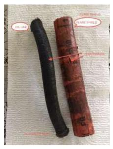
What was happening was that in normal operations with ram air cooling the engine, the oil was leaking on to the top of the oil cooler and then spread by airflow to the belly.
