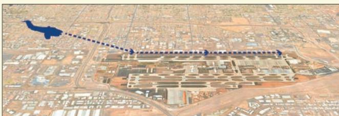
**VOR Orbits and Radial Flight** – These maneuvers are conducted on VORs, TACANs, and NDBs to ensure the integrity of the signal at various altitudes. They measure the signal's accuracy, strength, polarization, and modulation. The distance of the orbit is dependent upon the type of inspection being conducted, and some of those orbits can be as far as 70 miles from the facility.
