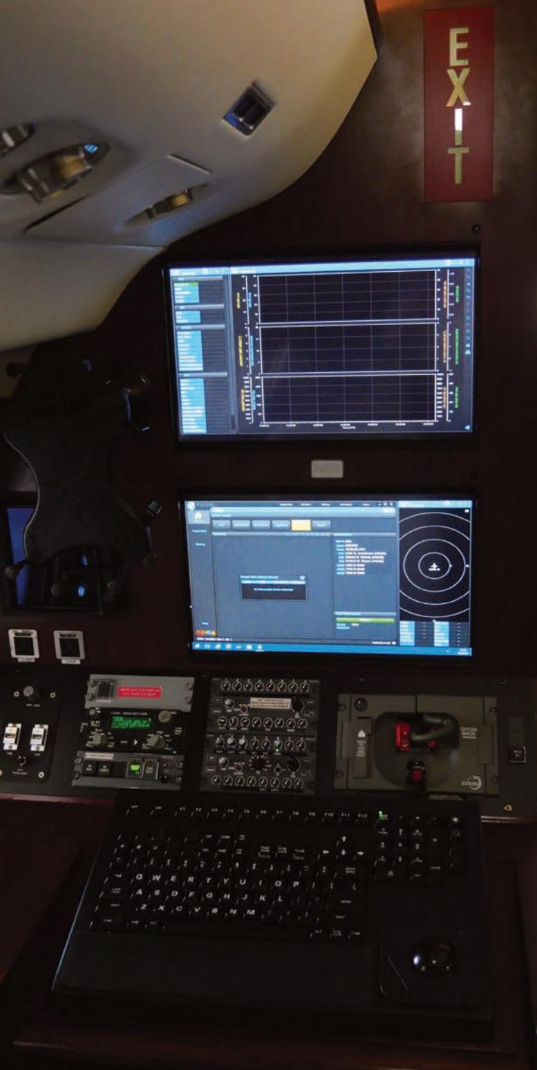
Today's flight inspection equipment is complex and specially developed to do its job.
