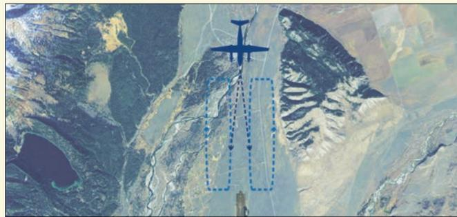
**Flight Inspection Low Approach** – This is often a test of the RNAV instrument approach procedure and the ILS. It is completed by a low approach 50 feet above the runway all the way to the opposite threshold. This ensures GPS database integrity and ILS signal accuracy. The flight inspection crew also uses this opportunity to inspect the entirety of the approach and runway lighting system.
