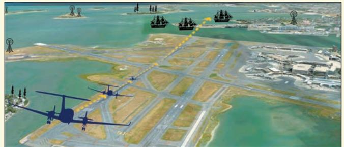
**Standard Instrument Departures (SID) and Standard Instrument Arrivals (STAR) Procedures** – These procedures are evaluated before publication to make sure each can be flown with varying navigation equipment capabilities,
