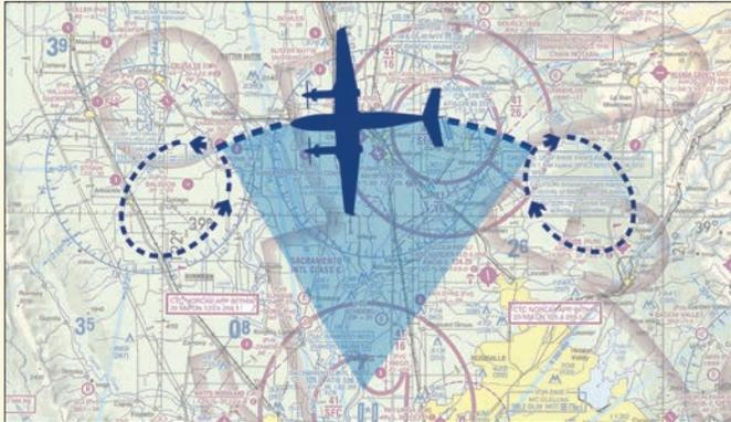
**Flight Inspection Holding Pattern** – This maneuver is specific to measuring the glideslope portion of an ILS and is typically conducted 1,500 feet above field elevation, from about 1-2 miles from the runway threshold. Of particular importance is that during this portion of the inspection, aircraft in the glideslope critical area during recording may interfere with the signal and result in a need to repeat the maneuver.
